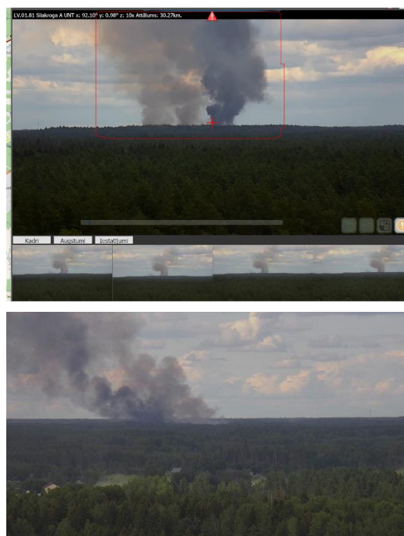
Figure 62. Remote Fire Detection and Monitoring System.
