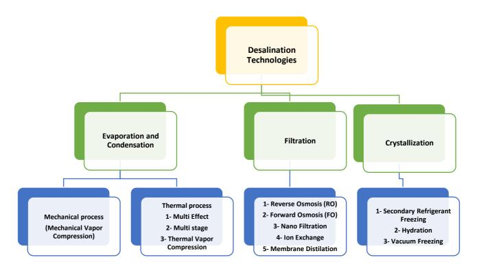
Figure 7: Classification of the desalination technologies according to the working principles
